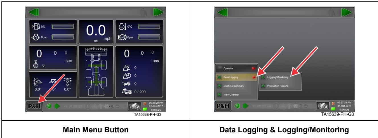
LINCS logging/monitoring menu access
