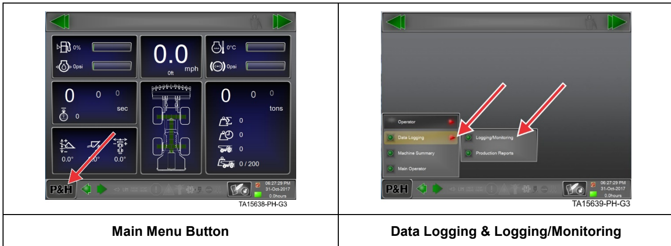
LINCS logging/monitoring menu access
