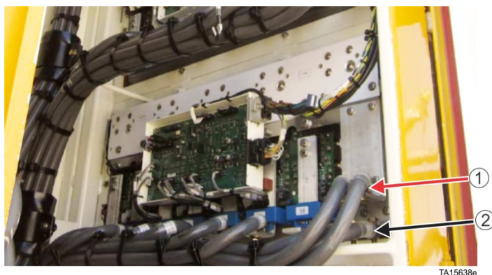
1) Positive bus bar, 2) Negative bus bar
