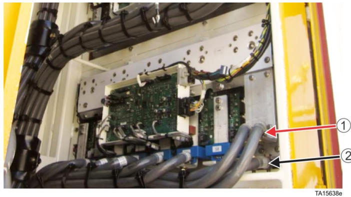
1) Positive bus bar, 2) Negative bus bar
